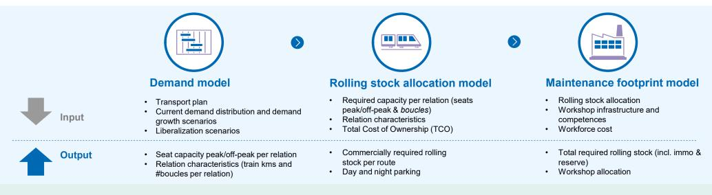
**Timetable Integrated Maintenance (TIM)** integrates in a smart way the maintenance in shifts to reduce downtime
